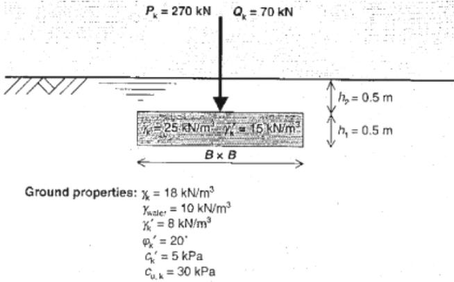
Under undrained conditions, the design bearing resistance may be calculated from:
