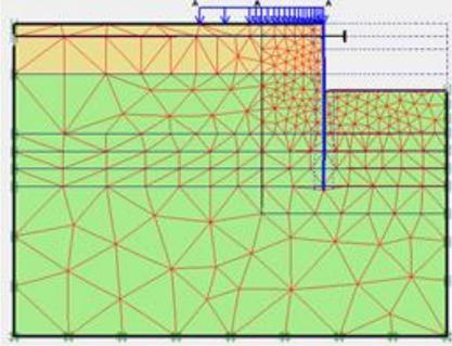
Fig. 7. (a) Hydraulic boundary condition and ground water head (equipotential lines) for FE analysis and (b) equilibrium water pressure distribution on active and passive sides of excavation
